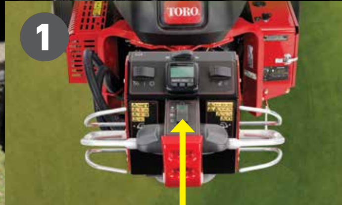
1 Set selector switch to Delayed Mode
